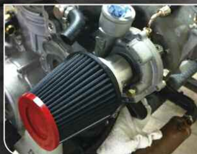
FLAME ARRESTOR #59-2040RR INSTALLED
