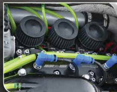
FLAME ARRESTOR #59-2045 INSTALLED
