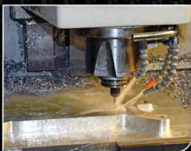
CNC filter mold fabrication
