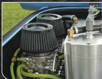
FLAME ARRESTOR #59-2046 INSTALLED
